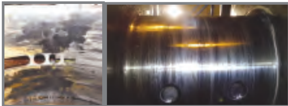
A burnt bearing shell (left) and severely damaged crank-pin (right) because of lubrication failure
