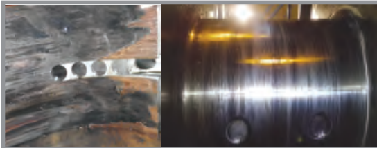
Severely damaged bearing shell (left) and crank-pin (right) because of lubrication failure
